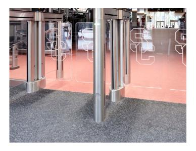
For the cardio and functional training areas, Gilman selected Ecore Performance Rally flooring. This 14.5mm product combines a 2.5mm wear layer with a 12mm shock-absorbing base layer and is engineered to absorb the impact force related to aggressive functional training.
